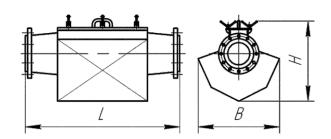
Designed for extracting ferro magnetic impurities from dry materials that are moved by pneumatic transport.
