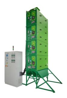
Intended for dry separation of mineral raw materials by electrical properties\* (usually for the separation of two non-conductive minerals).
