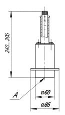
Designed for conducting high-quality express analysis of magnetic mineral flakes content in mineral raw material and for defining field characteristics, needed for carrying out magnetic separation of raw material.
