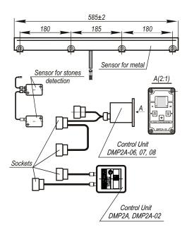
Designed for detecting ferromagnetic metallic as well as o.a.d. non-metallic(stones) objects (DMP2A-06).
